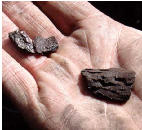
Scale washed out of FCAF N o .3. The scale shown was all removed by chemical action. No mechanical action was required. © M.Bane
